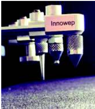
Steel Tip Groups Steel ball: 0.8 mm 1.8 mm 5.0 mm Steel Cone: 60°
