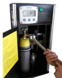
Casket with the SO 2 bottle and controller
