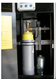
Bottle with SO 2 inside DosiCORR® ED unit
