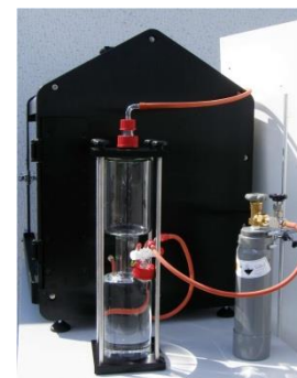
Front and side view of the glass cylinder for the manual gas dosing unit DosiCORR® MD
