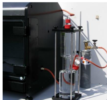
Front and side view of the glass cylinder for the manual gas dosing unit DosiCORR® MD
